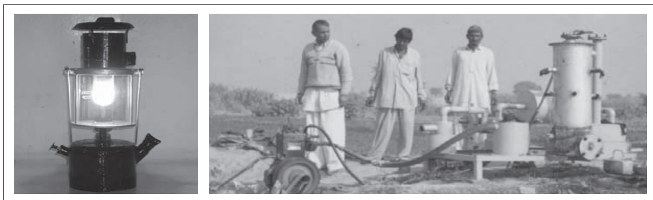
Figure 4 Ethanol-based lantern (left) and biomass gasifier (right)
